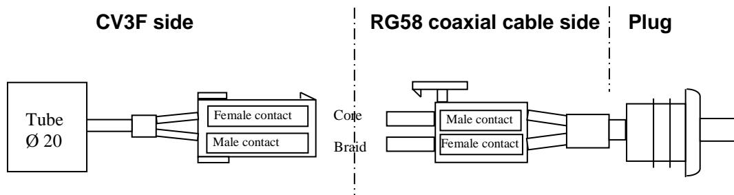
The plug at the end of the tube has a hole to allow the passage of coaxial cable RG58 and a small hole (1.5mm), sufficient to assure a natural weatherproofing and at the same time to stabilize the internal and external pressures on CV3F. During installation, care must be taken to ensure that this hole is not closed, and to be left in the same atmospheric pressure as the sensor itself.
